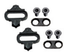
98A (52 g/pr) Cleat kit with improved mud clearance features. 4 degree float
